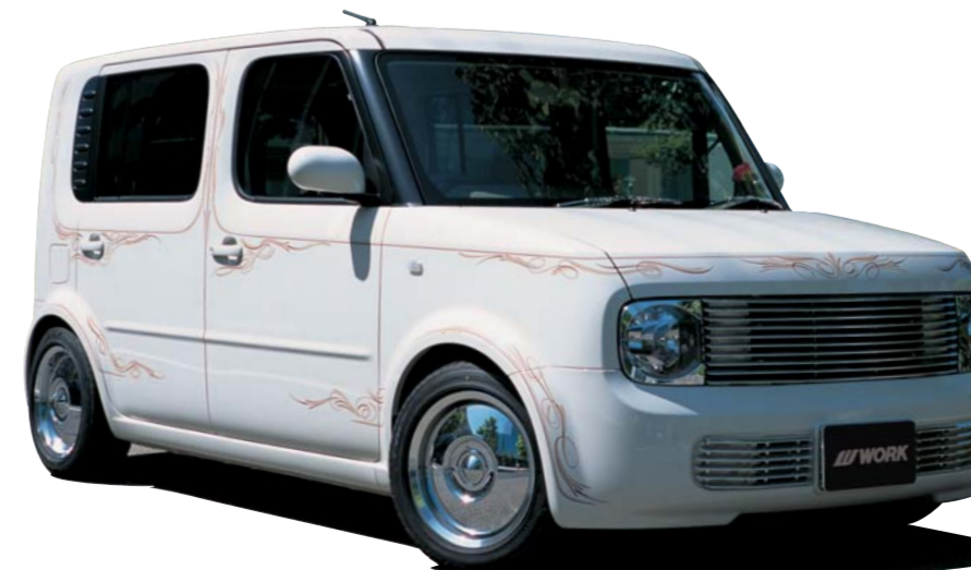
[SIZE] FRONT:15inch×6.5JJ OFFSET +48mm (A) TIRE:185/55-15 REAR:15inch×6.5JJ OFFSET +40mm (A) TIRE:185/55-15 COLOR:クロームメッキ (M) ※フェンダー加工
